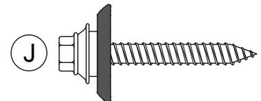
2 VIS DE 1 1/2 PO POUR TOITURE REQUISES AVEC RONDELLES POLYZIP
